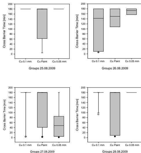
**Fig. 4** Box Plot graphics for the Cross Barrier Time of Cu 0.1 mm, Cu Paint and Cu 0.05 mm for each of the 4 days of testing.
